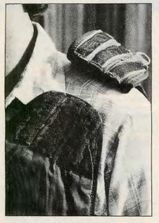
Shoulder detail illustrates vest attachment: first known Soviet use of hook-and-pile fasteners similar to U.S. Velcro. Note lack of neck protection.
